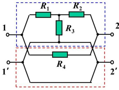
$$[Y_2] = \begin{bmatrix} \frac{1}{R_4} & -\frac{1}{R_4} \\ -\frac{1}{R_4} & \frac{1}{R_4} \end{bmatrix}$$
